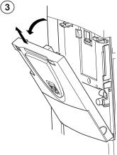
Using a screwdriver, press down on the catch and pull to release the lefthand part of the control front panel
