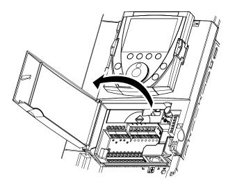
To access the control terminals, open the cover on the control front panel
