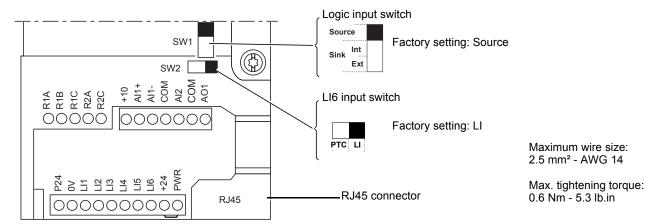
Note: The MT Series is supplied with a link between the PWR and +24 terminals.
