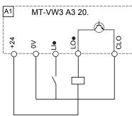
Switch in "Source" position and use of an external +24 VDC source
