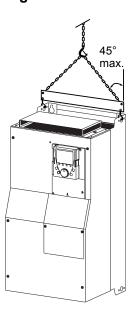
MT Series drives up to ratings MT220 and MT425 can be removed from their packaging and installed without a handling device.
