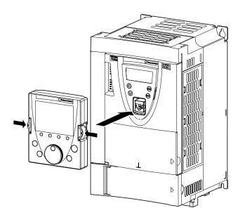
The graphic keypad can be connected or disconnected with the power on. Before disconnecting it, drive control via the display terminal must be disabled (refer to the programming manual).
