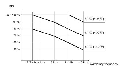
For intermediate temperatures (e.g. 55°C [131°F]), interpolate between 2 curves.
