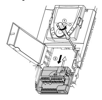
To make it easier to wire the drive control section, the control terminal card can be removed.
