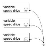
Check whether the resistance to the protective ground is one ohm or less. Connect a number of variable speed drives to the protective ground, as shown in the diagram (see left). Do not lay protective grounding cables in a loop or in series.
